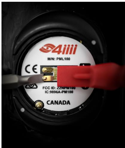
Then, place an upside-down (+ terminal down) battery into the pod so that it touches both of the battery contacts for a few seconds before reinstalling the battery in the correct orientation. This will remove any residual charge.
