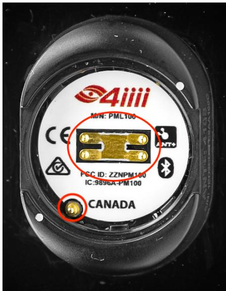
If it looks like the large rectangular one is flat against the bottom, use a jeweler's screwdriver or similar tool to very gently lift the ends of the prongs 1mm off the bottom of the pod, so that they press against the battery more firmly. Make sure to hold down the center of the battery tab while lifting the prongs.
