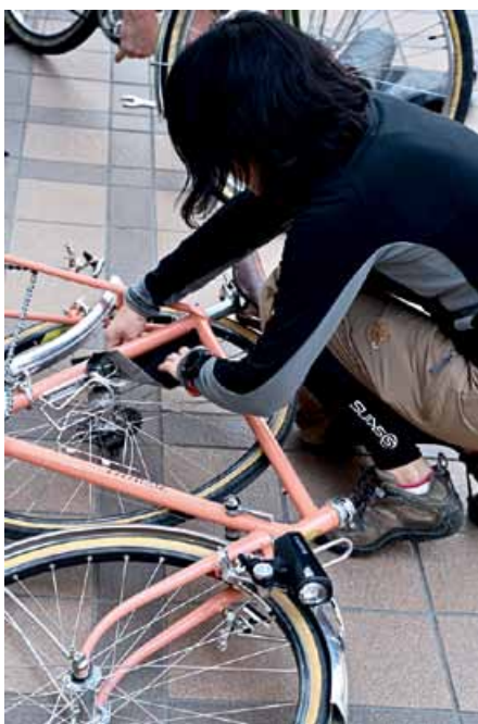
11. She places the bike onto the rear wheel and wraps a piece of padding around the seat tube. No other padding is used, yet the bike remains scratch-free after many train trips. Natsuko explains: "If you pack carefully, there will be few places where the parts touch and can scratch each other."
