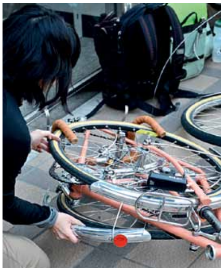
14. The rear fender goes onto the rear wheel. The stays are threaded into the spokes, so they don't scratch the frame.
