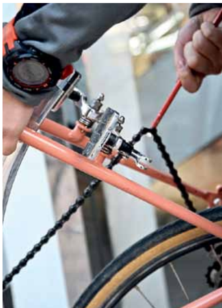
10. Natsuko removes the rear wheel and hooks the chain onto its hanger, using the Allen wrench. No dirty fingers here!
