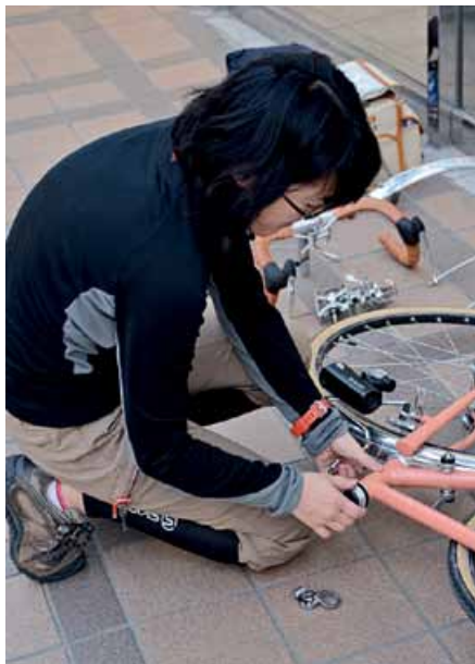
12. Natsuko unscrews the headset and removes the fork. The headset parts go back onto the fork, so they don't get lost.
