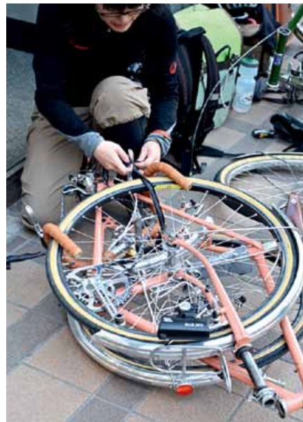
15. Straps keep the parts from rattling.
