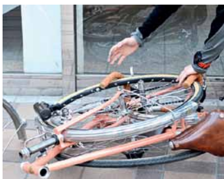
13. She places the fork, with the front wheel installed, on the frame and wraps the handlebars around the package.
