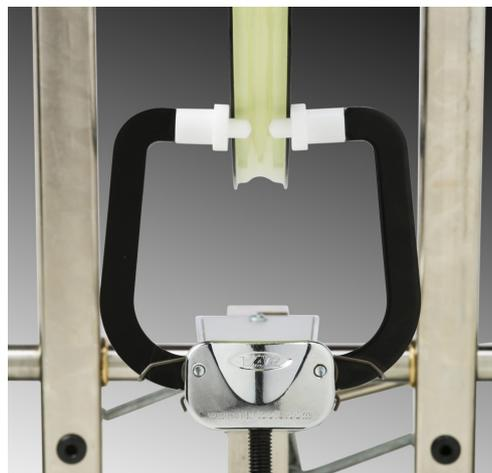
**2. Regularly spray VAR NL-76000 on the horizontal guides. It eases the uprights movements and prevents the bushings from premature wear.**
