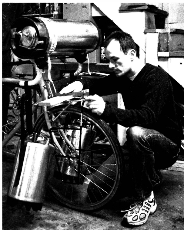
Fig. 1: Weights on the handlebars simulated the loads fed into the fork by road irregularities (Fork 1 shown).
