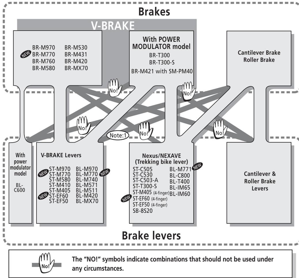
Note 1: This combination will not provide the sufficient amount of braking force.
