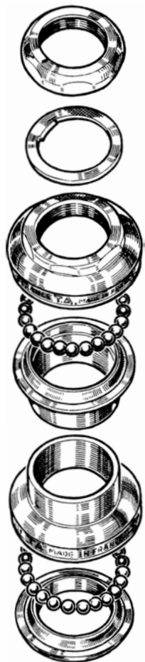
Opposite : left. Headset components in order of assembly. From bottom to top, crown race, steel balls, bottom frame race, upper frame race, steel balls, adjusting race, adjusting washer and locknut.
