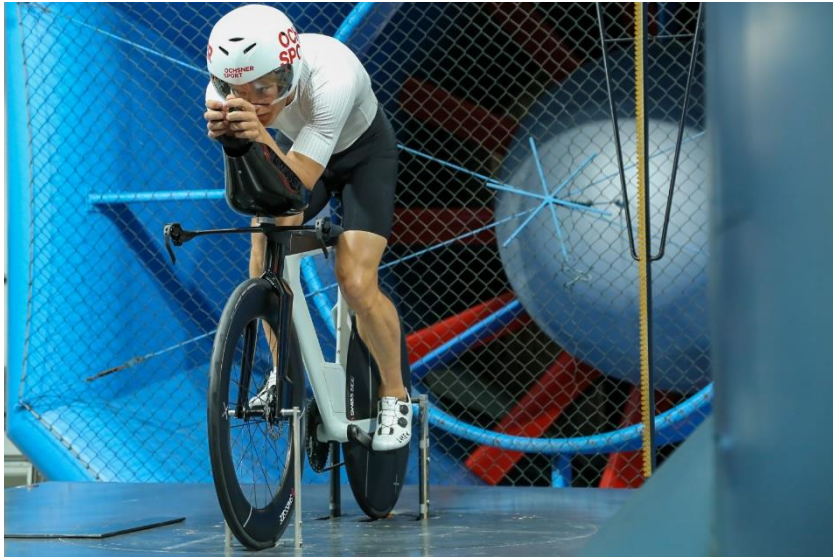
Figure 5: One athlete with an AERO Tri Suit prototype in the full-size wind tunnel.
