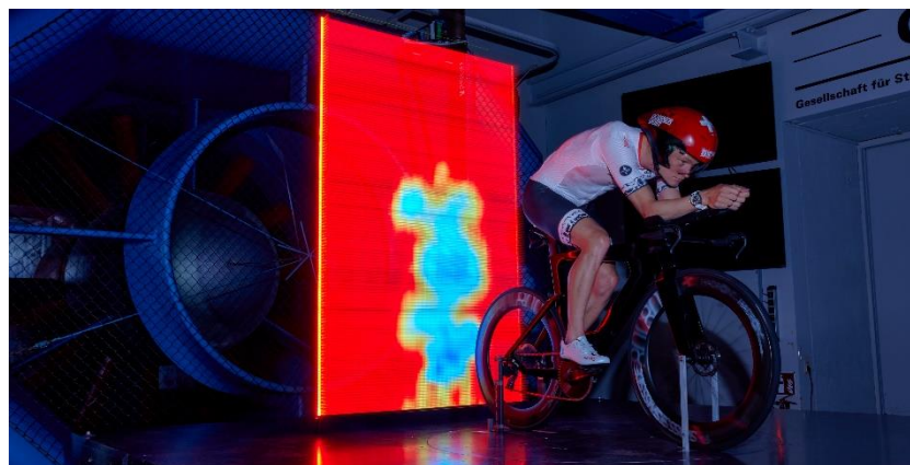
Figure 10: Aerodynamic measurements in a full-size wind tunnel on athlete. The red zone indicates no losses (100% total pressure). The darker the blue, the more the losses/aerodynamic drag.
