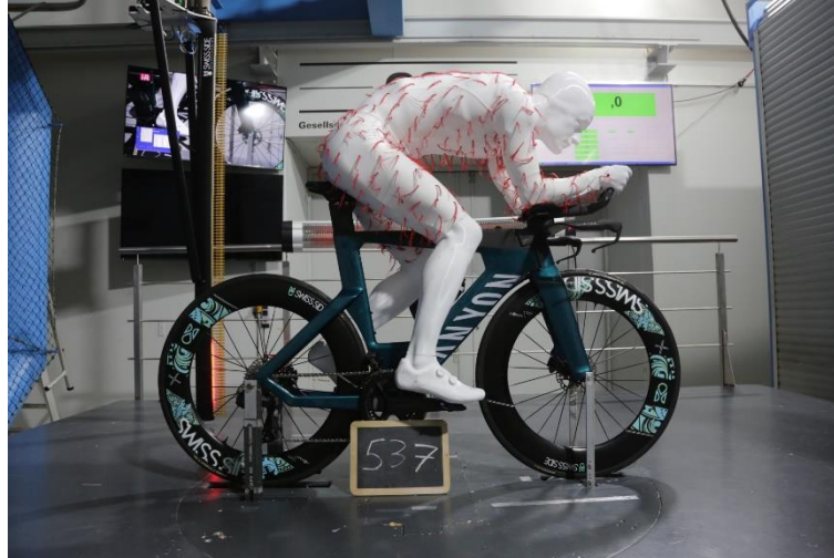
Figure 12: Time Trial mannequin with the chicken suit in the wind tunnel
