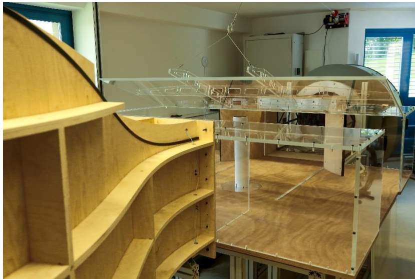
Figure 3: General image of the Swiss Side wind tunnel while fabric testing.
