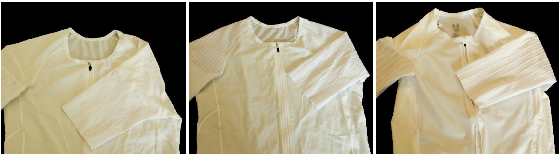
Figure 9: AERO Tri Suit prototypes with different fabrics on arms and shoulders.
