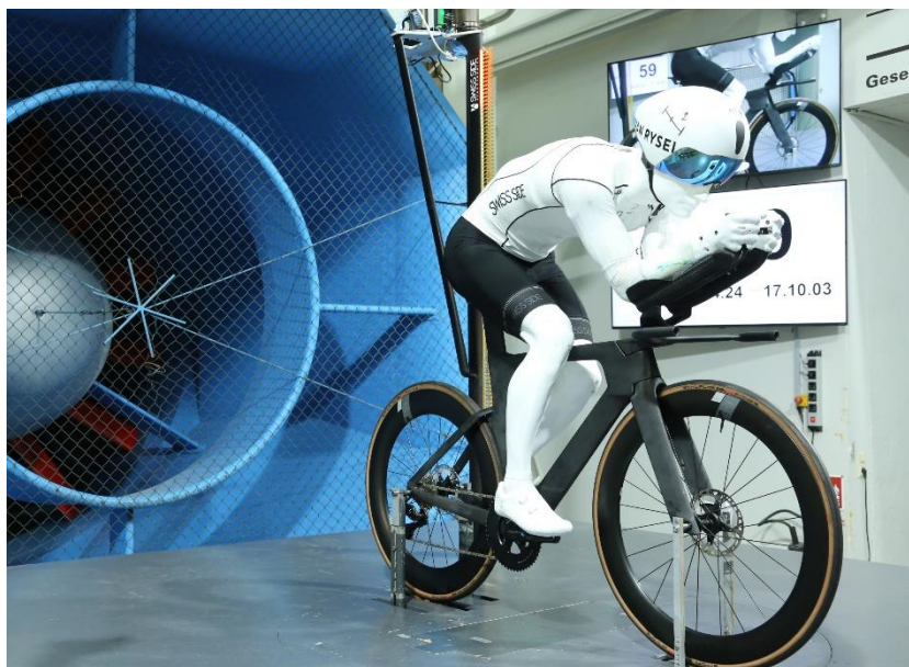
Figure 4: Time Trial mannequin testing with an AERO Tri Suit prototype in the wind tunnel.
